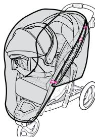
Attach raincover with hook and loop tape and snaps as shown.
